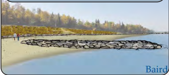
REACH 2: SOUTH CONCEPTUAL SKETCH OF ROCK GROYPNE, BEACH NOURISHMENT & TOE/SLOPE PROTECTION
