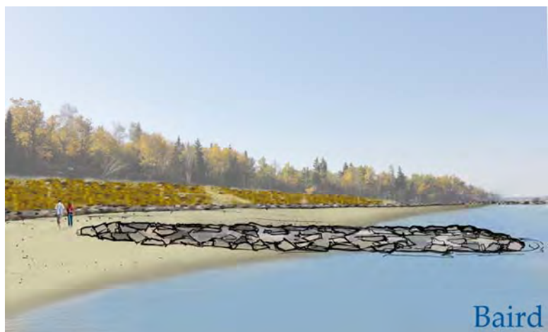
Figure 5.1 Example of Rock Groyne, Beach Nourishment, Toe Protection and Slope Re-grading and Vegetation
