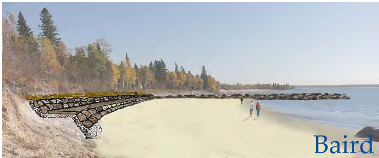
Figure 5.9 Example Boardwalk Incorporated into Toe Protection
