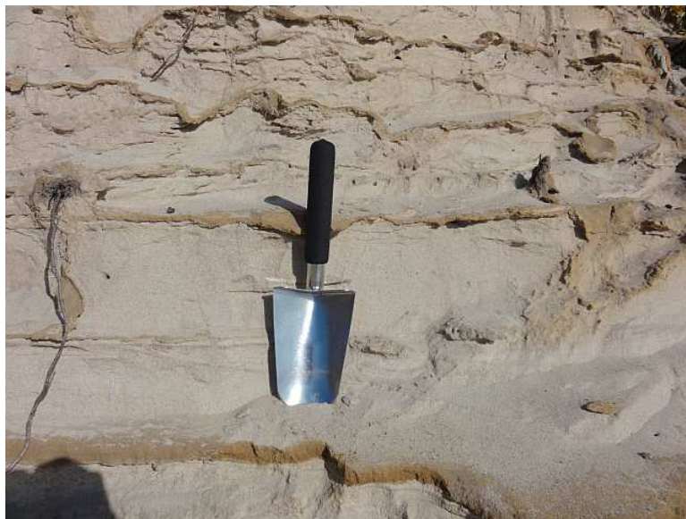
Figure 2.6 Sediment Sampling Shovel
